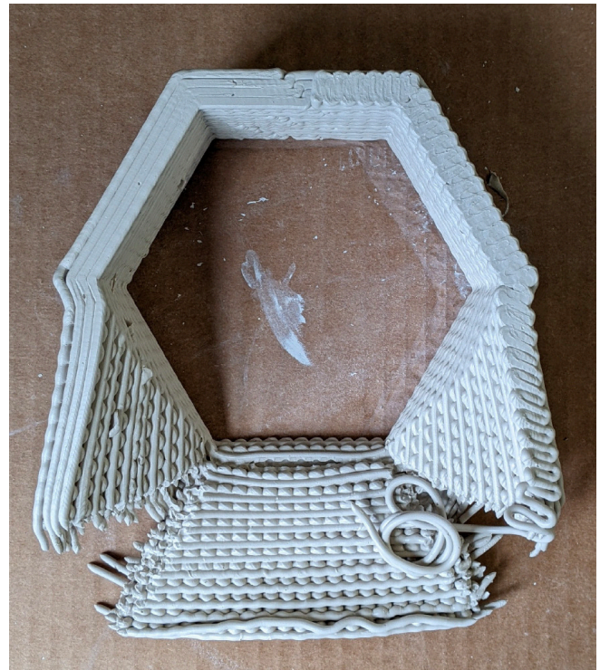
Figure 3. Printed studies testing material weave and strength.
